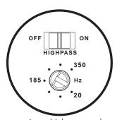
trol counterclockwise while listening for bottoming. You are lowering the crossover point, which means that more bass signal is being sent to the speakers. If bottoming is detected, Rotate FRONT input sensitivity control counterclockwise until it is eliminated and/or rotate the FRONT highpass crossover control clockwise to raise the crossover point.
